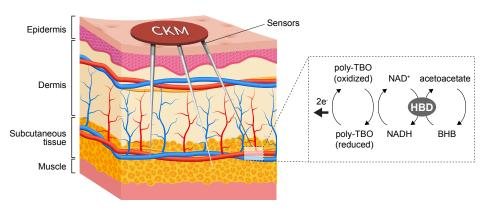
β-hydroxybutyrate dehydrogenase (HBD) reduces NAD+ into NADH and oxidizes BHB to acetoacetate. NADH is in turn oxidized at the electrode surface to generate a current proportional to BHB concentration.
